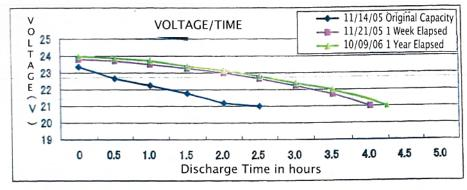
3. After one year elapsed time of daily usage battery remained at 84% capacity. Estimated battery recovery time is 2 years (4.5 hours).
